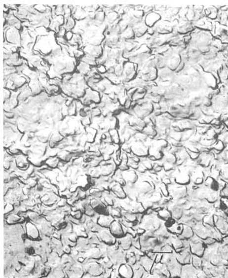
Fig. 8. Globular forms of the surface of the central part of gold cover of drusy cavities from the Overlying Helena Vein — 5th horizon. Two-degrees replica of natural surface, magnif. 5750 X. Photo by M. Harman.
