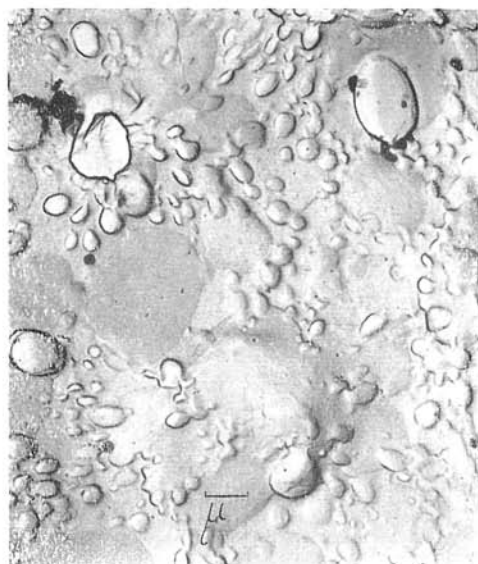
Fig. 9. Two generations of globular forms on the surface of the central part of the gold cover from drusy cavities of the Overlying Helena Vein — 5th horizon. Two-degrees replica of natural surface, magnif. 5750 X. Photo by M. Harman.
