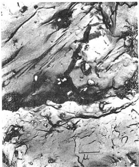
Fig. 3. Finely dispersed porphyry electrum, mostly concentrated in zones of inhomogeneity of grey vein quartz from the Helena Vein. Two-degrees replica of natural fracture surface, magnif. 9250 X. Photo by M. H a r m a n.
