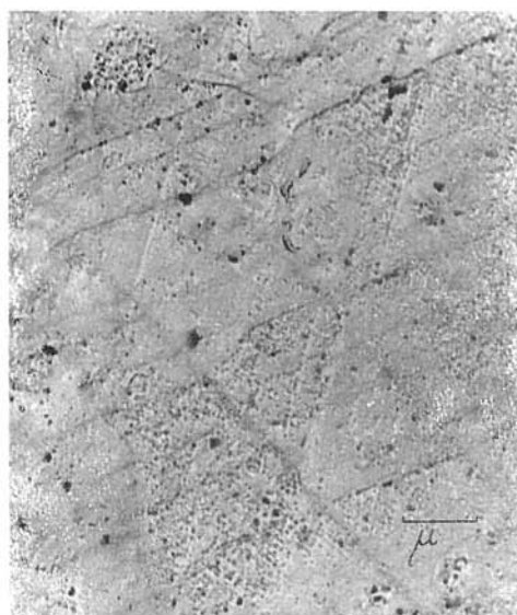
Fig. 10. Porous ultramicrostructure with motives of isosceles triangles from peripheral parts of the gold cover from drusy cavities of the Overlying Helena Vein — 5th horizon. Two-degrees replica of natural surface, magnif. 9250 X. Photo by M. Harman.
